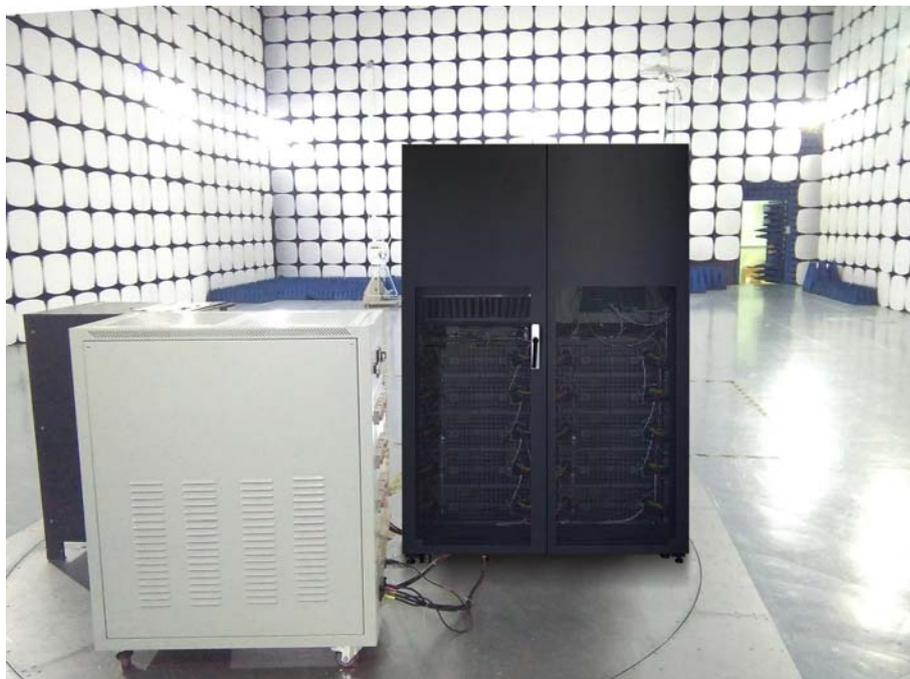
16.3. Photo of Electrostatic Discharge Test
